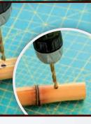
5. When you look inside the bamboo, you'll see a solid piece of wood at each joint. Use the paddle bit to drill out that wood at each end. You should be able to see all the way from one end to the other when you're done.
